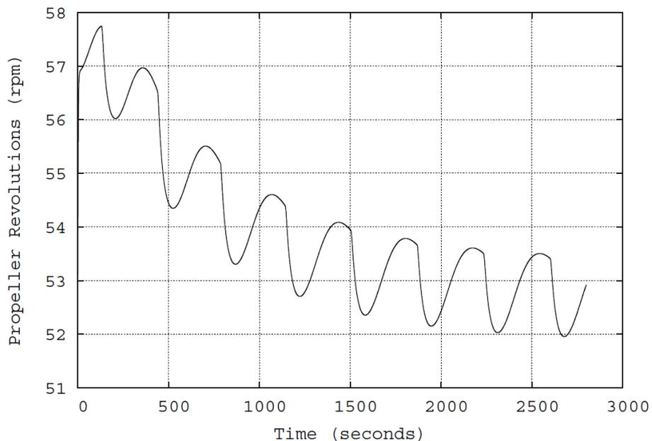
Figure 2: Variation of propeller speed with time during a 20/20 zigzag manoeuvre
