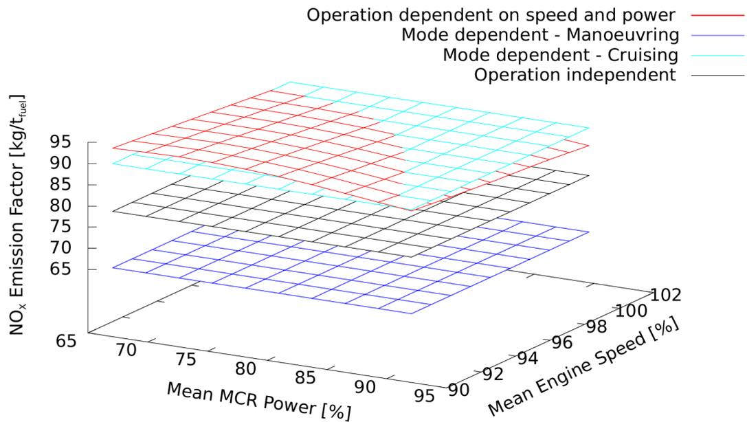
Figure 3: Variation in NO<sub>x</sub> emission factor with engine running conditions.
