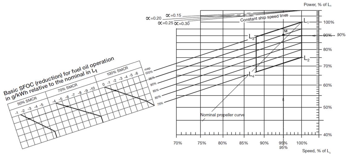
Figure 1: calculation of SFOC from MCR position [4]
