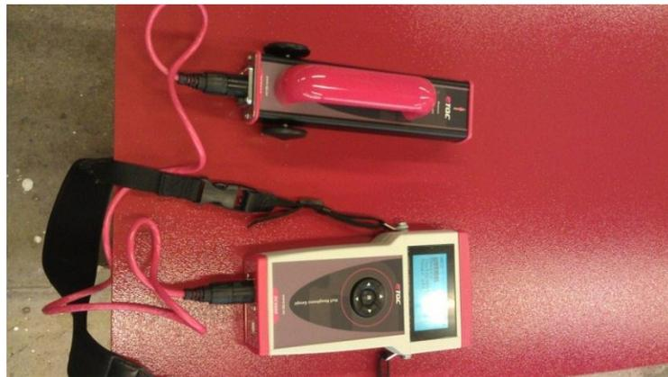
Figure 8: TQC Hull Roughness Gauge.
