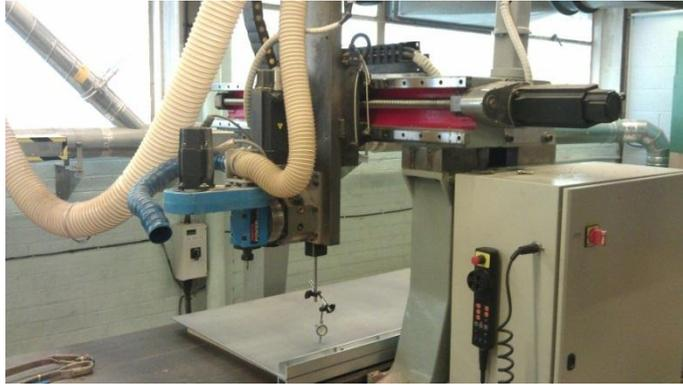
Figure 2: Checking the flatness of the plates.
