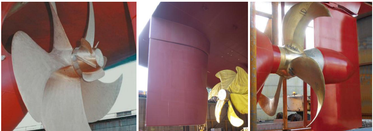
Figure 3: PBCF (left) (Hansen et al., 2011), Asymmetric Rudder (centre) and Rudder Bulb (right) (Becker Marine Systems)
