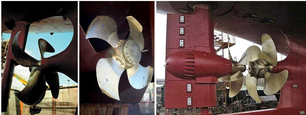
Figure 2: Kappel (left), CLT Propellers (centre) (Gennaro & Gonzalez-Adalid, 2012) and CRPP (right) (Kluijven, et al.)
