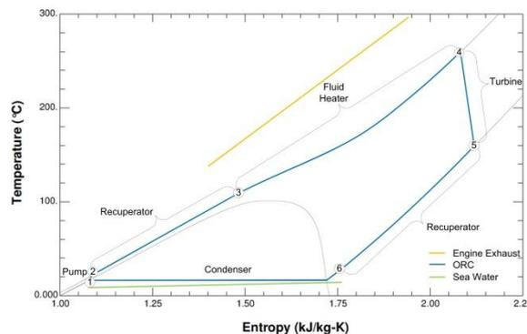
Figure 3 - SORC: Temperature-Entropy Diagram
