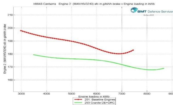
Figure 8. Diesel engine Sfc with and without the SORC system
