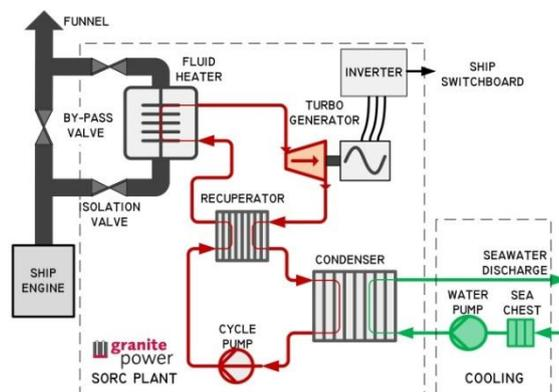
Figure 1 – SORC Schematic
