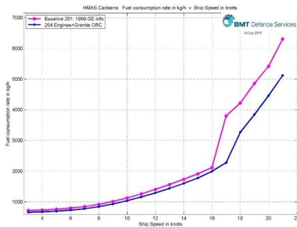
Figure 9. Comparative fuel consumption rates
