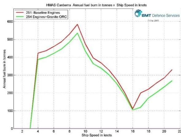
Figure 10. Relative fuel consumption at each speed
