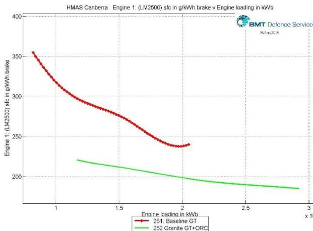
Figure 7. GT engine Sfc characteristic with and without the SORC system
