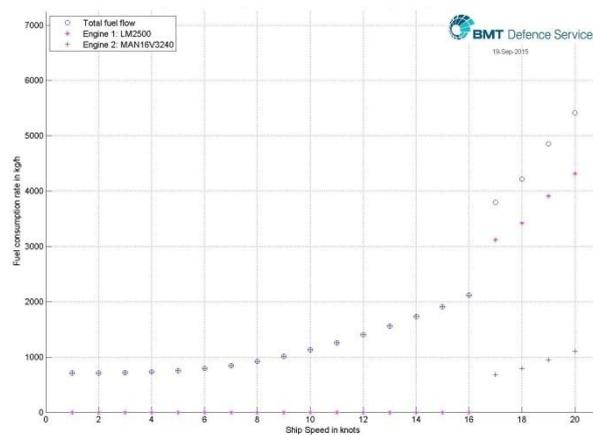
Figure 6. HMAS Canberra baseline total fuel consumption rate versus ship speed
