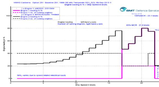
Figure 5. HMAS Canberra estimated engine load for the whole speed range
