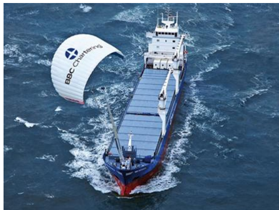
Figure 6 - A towing kite in action ( www.skysails.info )
