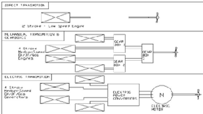
Figure 1: The different machinery topologies that were examined.
