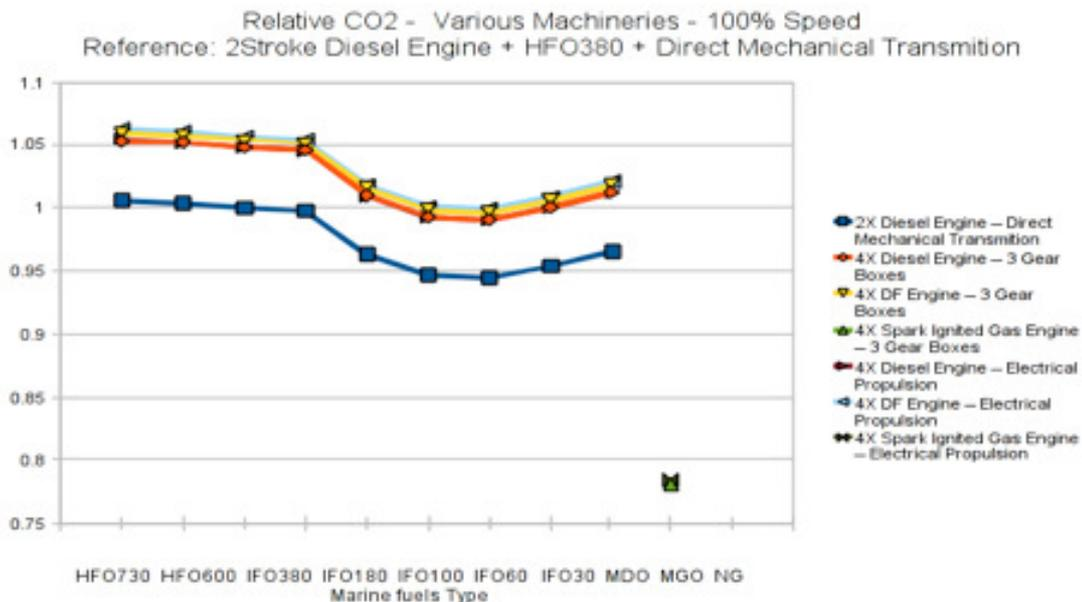
Figure 2: Relative CO<sub>2</sub> emissions reduction of different fuel and machinery arrangements for a panamax container carrier at 100% MCR with Gas engines running in diesel mode.
