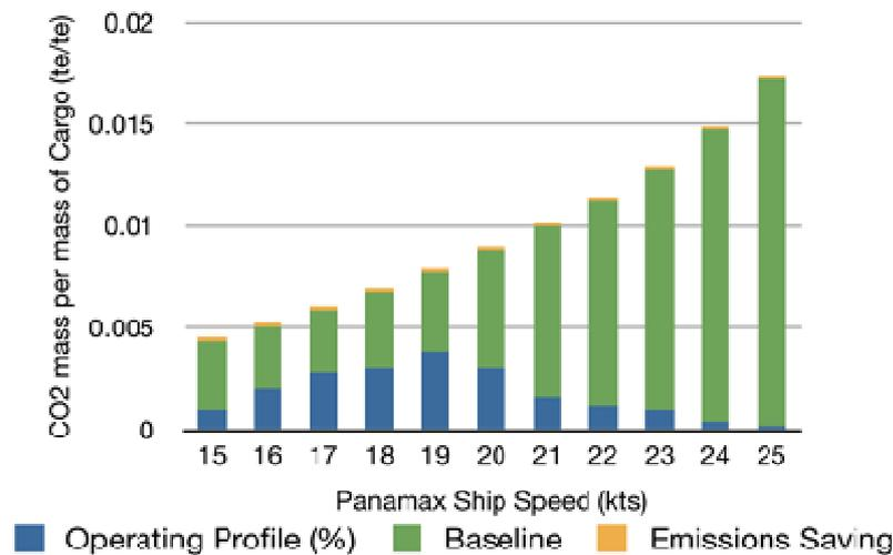
Figure 7: Carbon dioxide emissions for a panamax container carrier with LNG auxiliary power at different operating speeds.
