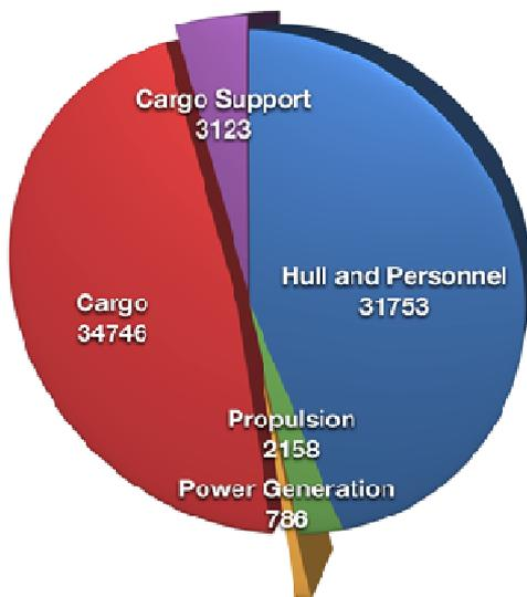
Figure 6: Panamax container carrier with LNG auxiliary power retrofit mass breakdown.
