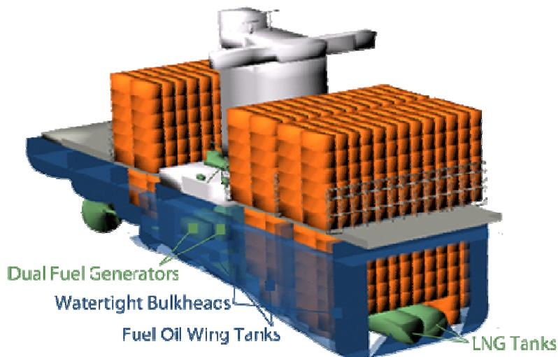
Figure 4: Potential LNG tank arrangement for auxiliary power on a panamax container carrier.
