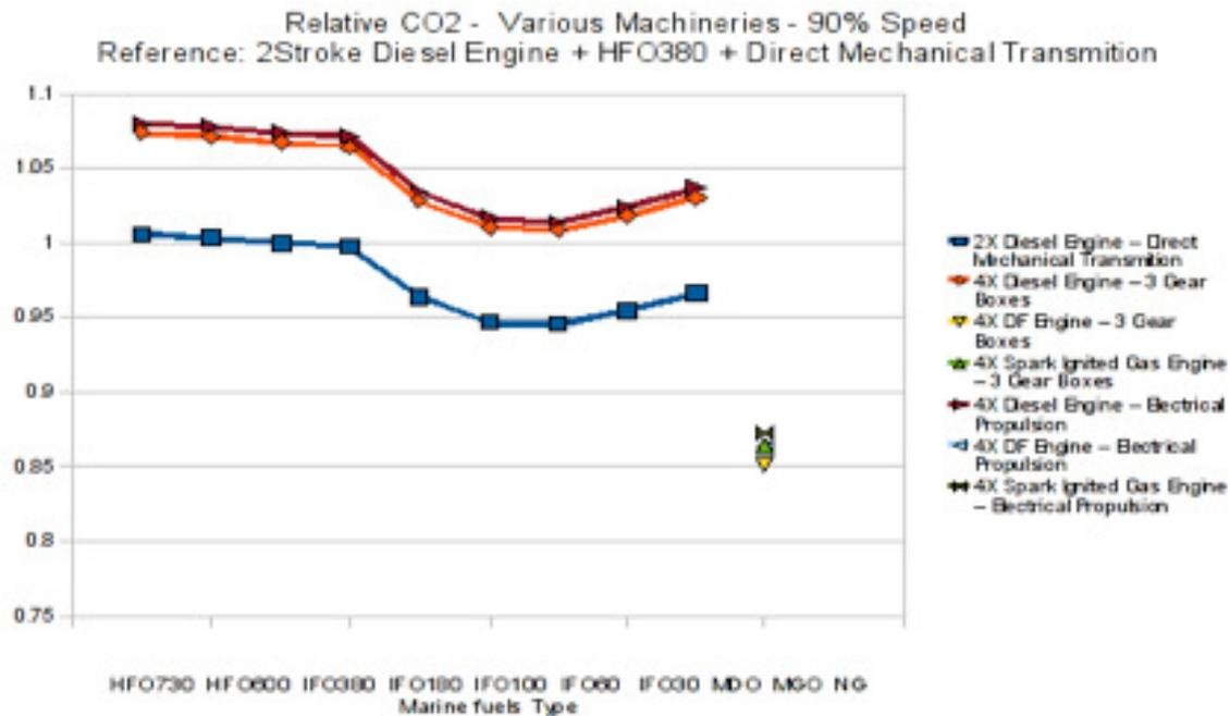
Figure 3: Relative CO<sub>2</sub> emissions reduction of different fuel and machinery arrangements for a panamax container carrier at 75% MCR.
