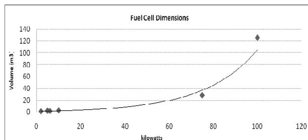
Figure 8: Fuel Cell total dimensions as function of power
