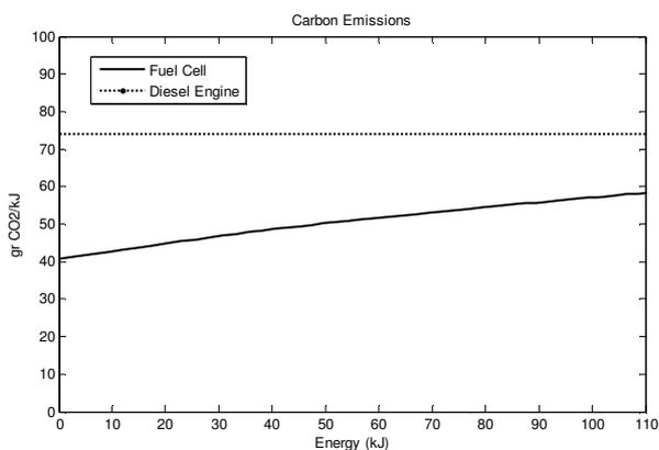
Figure 6: Calculated CO<sub>2</sub> Emissions per energy unit
