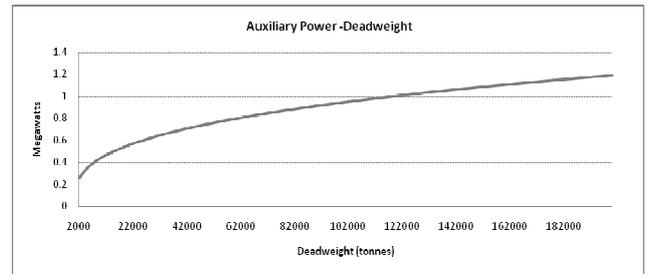
Figure 2: Calculation of Auxiliary Power demand on board
