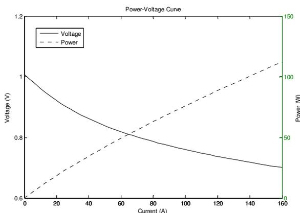
Figure 5: Fuel Cell Voltage and Power curves
