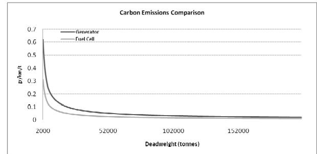
Figure 12: CO<sub>2</sub> emissions comparison between Fuel Cell and marine diesel engine generator as a function of cargo deadweight
