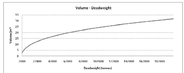
Figure 4: Required volume for a marine diesel engine generator as a function of cargo deadweight
