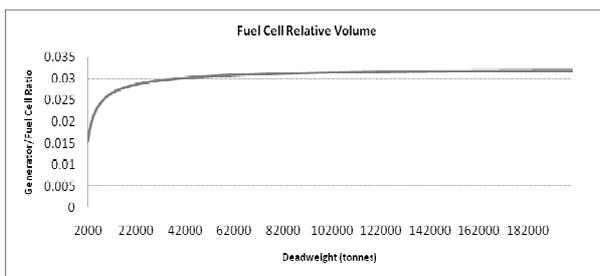
Figure 11: Relative volume of Fuel Cell that can be installed for the volume required of a marine diesel engine generator
