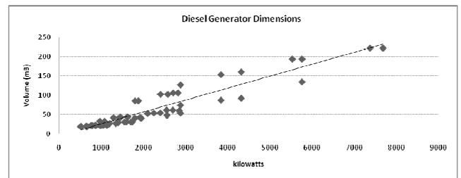
Figure 3: Estimation of the dimensions required for a marine diesel engine generator
