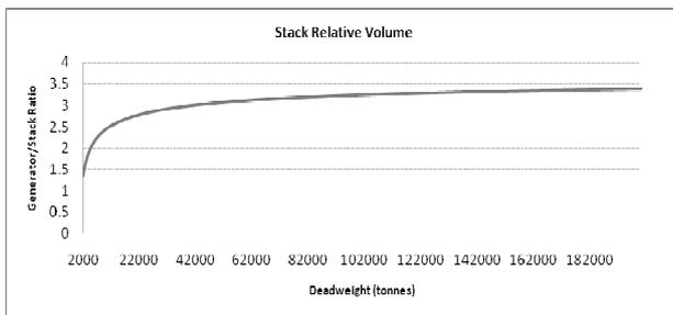
Figure 10: Relative volume of Fuel Cell stack that can be installed for the volume required of a marine diesel engine generator
