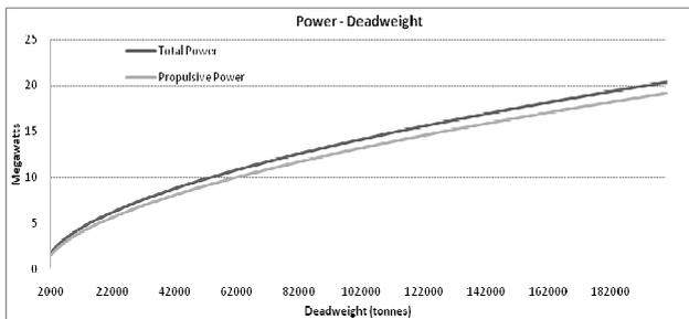
Figure 1: Calculation of Total Power and Propulsive Power for cargo deadweight
