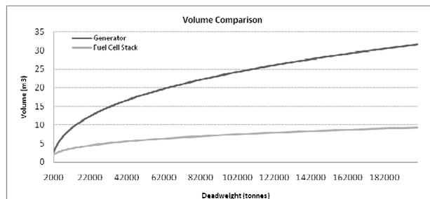
Figure 7: Comparison between Fuel Cell Stack and marine diesel engine dimensions as function of cargo deadweight
