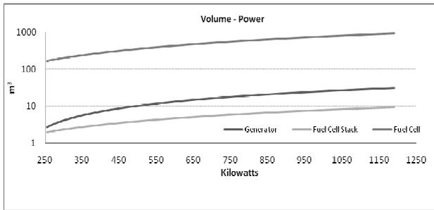
Figure 9: Comparison between Fuel Cell, Fuel Cell Stack and marine diesel engine dimensions
