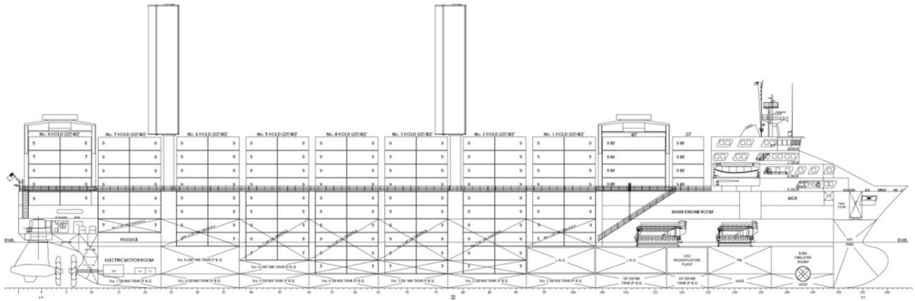
Figure 4: General arrangement profile view of fast sail assisted feeder container ship
