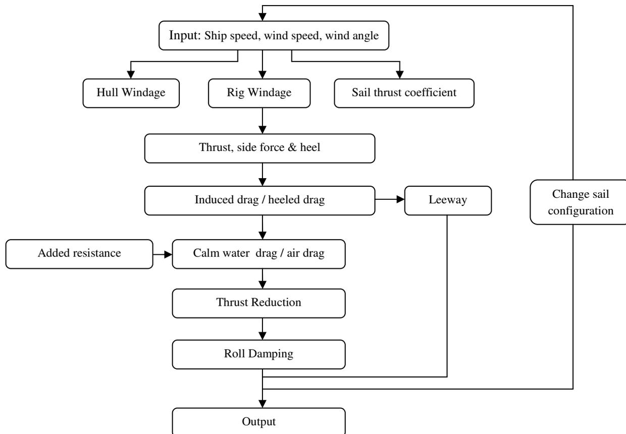
Figure 3: Flowchart summary of performance prediction program used to calculate sail thrust
