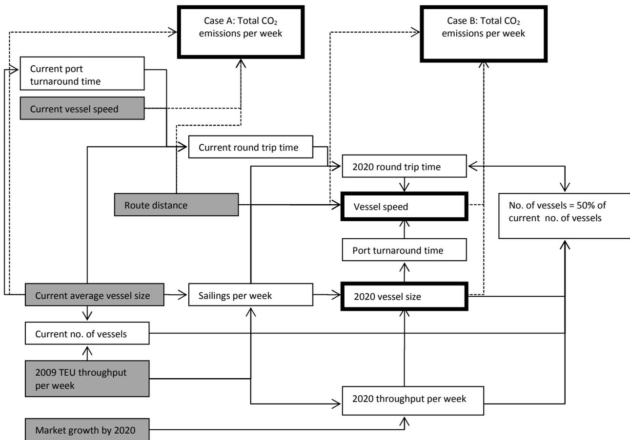
Figure 2: Flow chart used to determine the required ship capacity and speed for a particular route (shaded boxes represent process inputs, bold edged boxes outputs, and other boxes intermediate steps)
