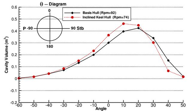
Figure 17: Comparison of cavity volume
