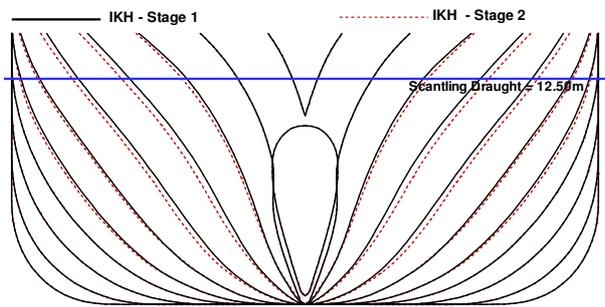
Figure 9: Comparison of fore body plans on level trim condition
