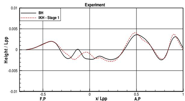
Figure 8: Comparison of wave cuts measured at  $y/L_{pp}=0.11$
