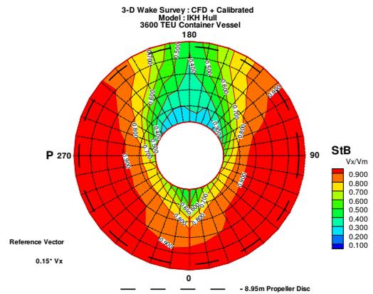
Figure 15: Wake distribution of the IKH from CFD-calibrated
