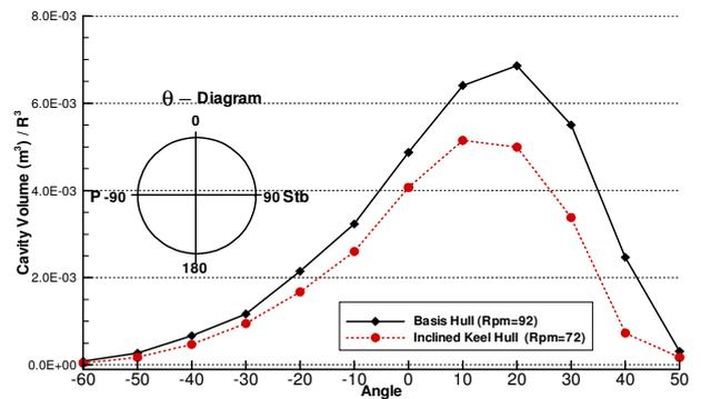
Figure 18: Comparison of non-dimensional cavity volume
