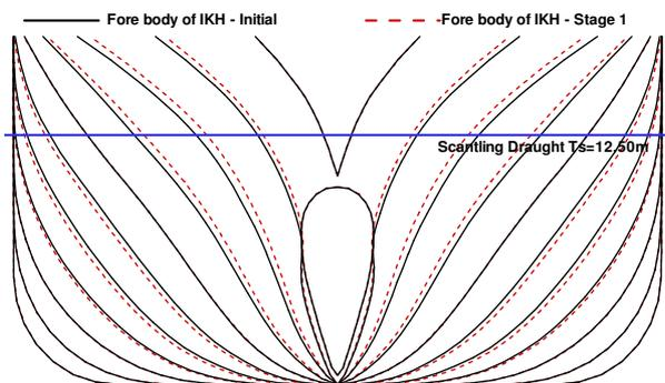
Figure 4: Comparison of fore body plans on level trim condition
