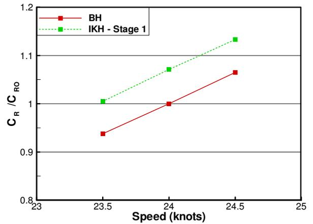
Figure 7: Comparison of residual resistance coefficients ( $C_{R0}$  represents the residual resistance of the BH at the design speed)
