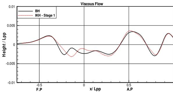
Figure 6: Comparison of wave cuts measured at  $y/L_{pp}=0.11$
