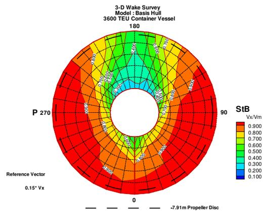
Figure 13: Wake distribution of the BH from experiment
