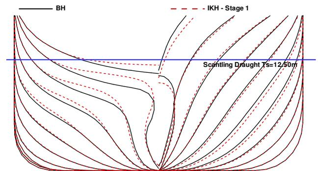
Figure 5: Comparison of body plans on level trim condition
