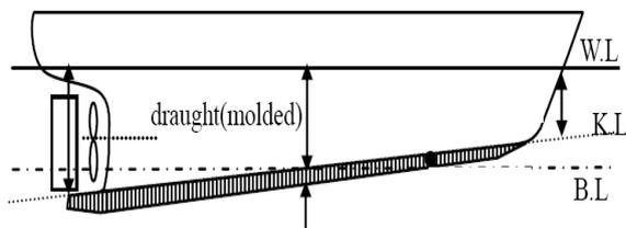
Figure 1: Configuration of the Inclined Keel Hull
