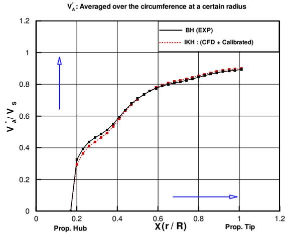
Figure 16: Comparison of the circumferential mean wake distribution
