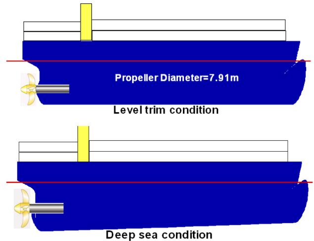
Figure 2: Definition of the Inclined Keel Hull (Upper figure represents the BH and Lower figure represents the IKH)
