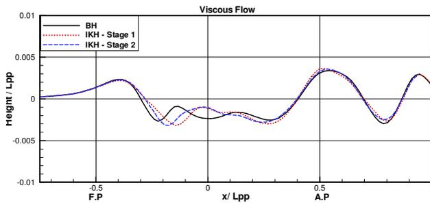
Figure 12: Comparison of wave cuts measured at  $y/L_{pp}=0.11$
