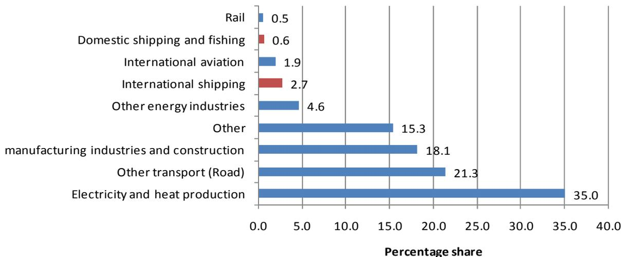
Figure 1: Emissions of CO<sub>2</sub> from shipping compared with global emissions from other industries (2007) (Buhaug et al 2009).
