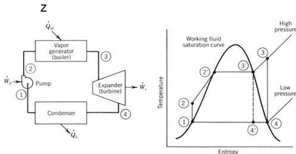
Figure 3: Steam Cycle with superheating 3'-3 and one expander (turbine).
