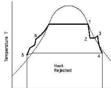
Figure 4: Nuclear steam cycle using two expanders, with reheating (2-3) between high pressure (HP) (1-2) turbine and low pressure (LP) turbine (3-4) and preheating (5-6)
