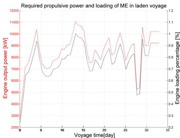
Figure 5: Simulated engine loading and engine power output during the examined laden voyage
