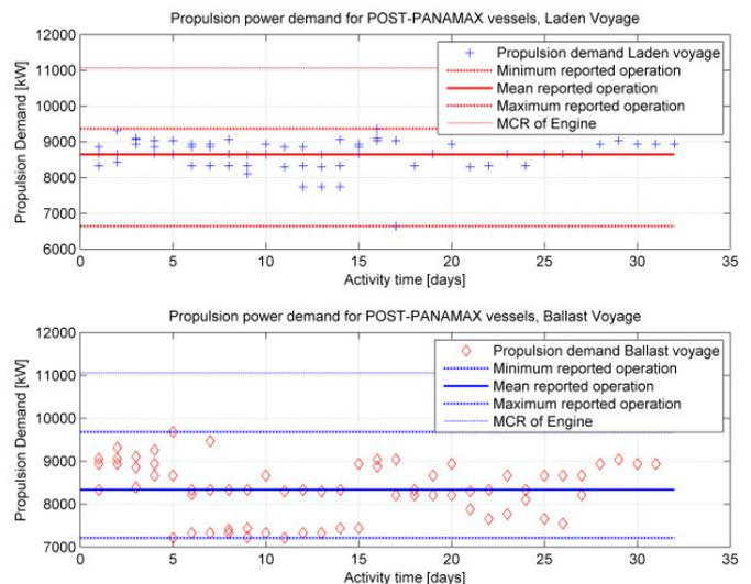
Figure 2: Engine loading based on noon-report data as edited in the work of Dedes, et al. (2011).
