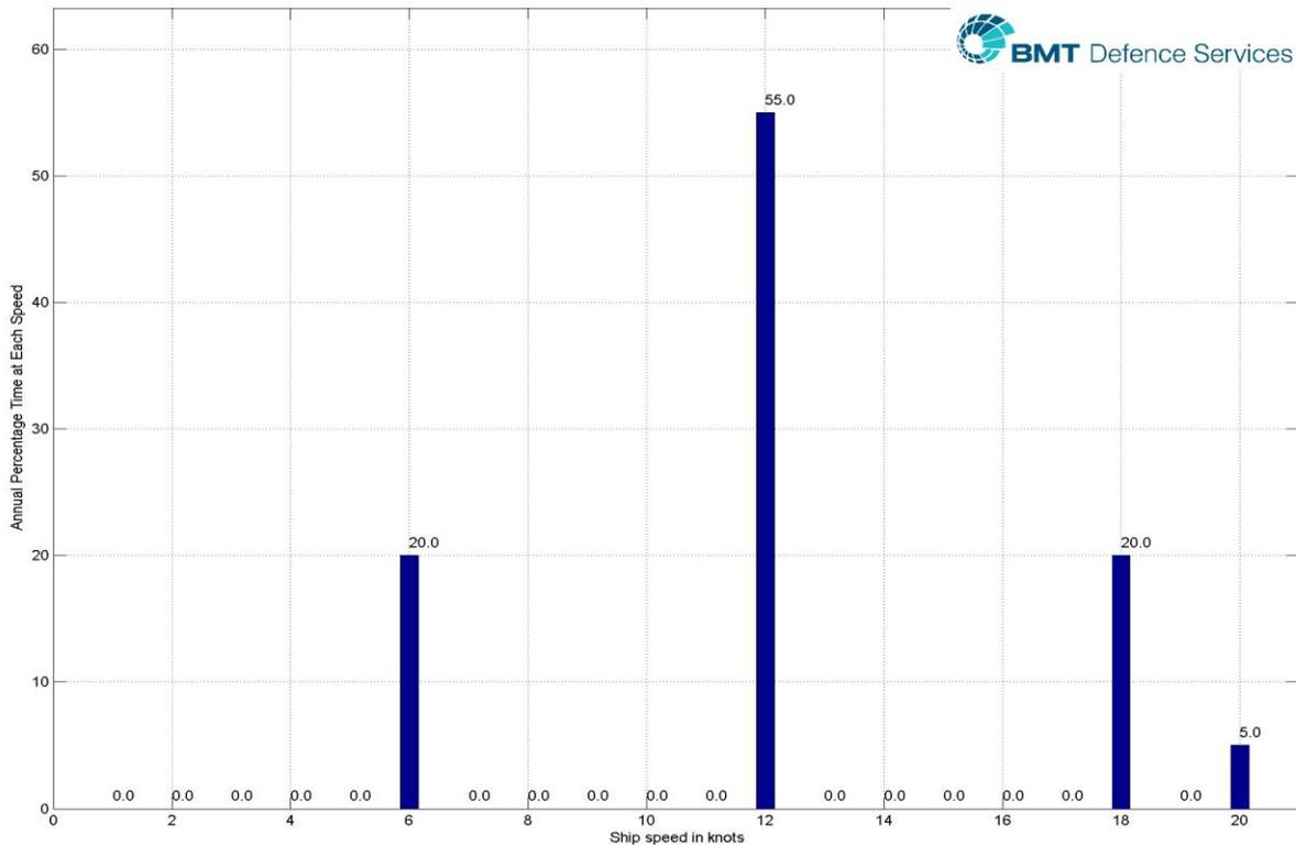
**Figure 1: Ship Speed-Time Operating Profile**
