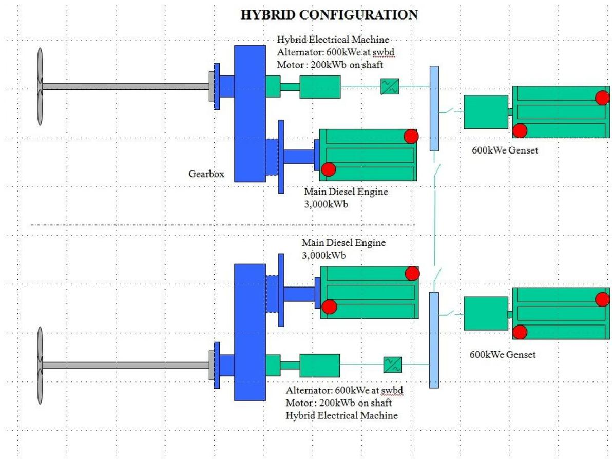
**Figure 3: Hybrid Arrangement**
