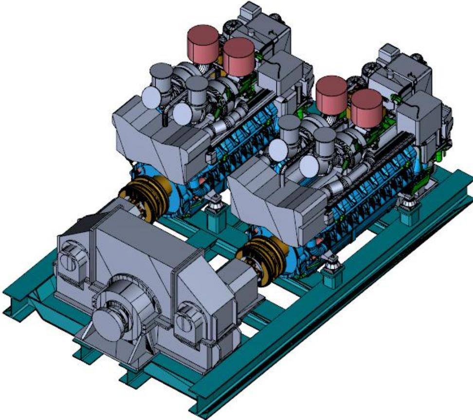
**Figure 1: The Renk-MTU Power-Pack Arrangement**
