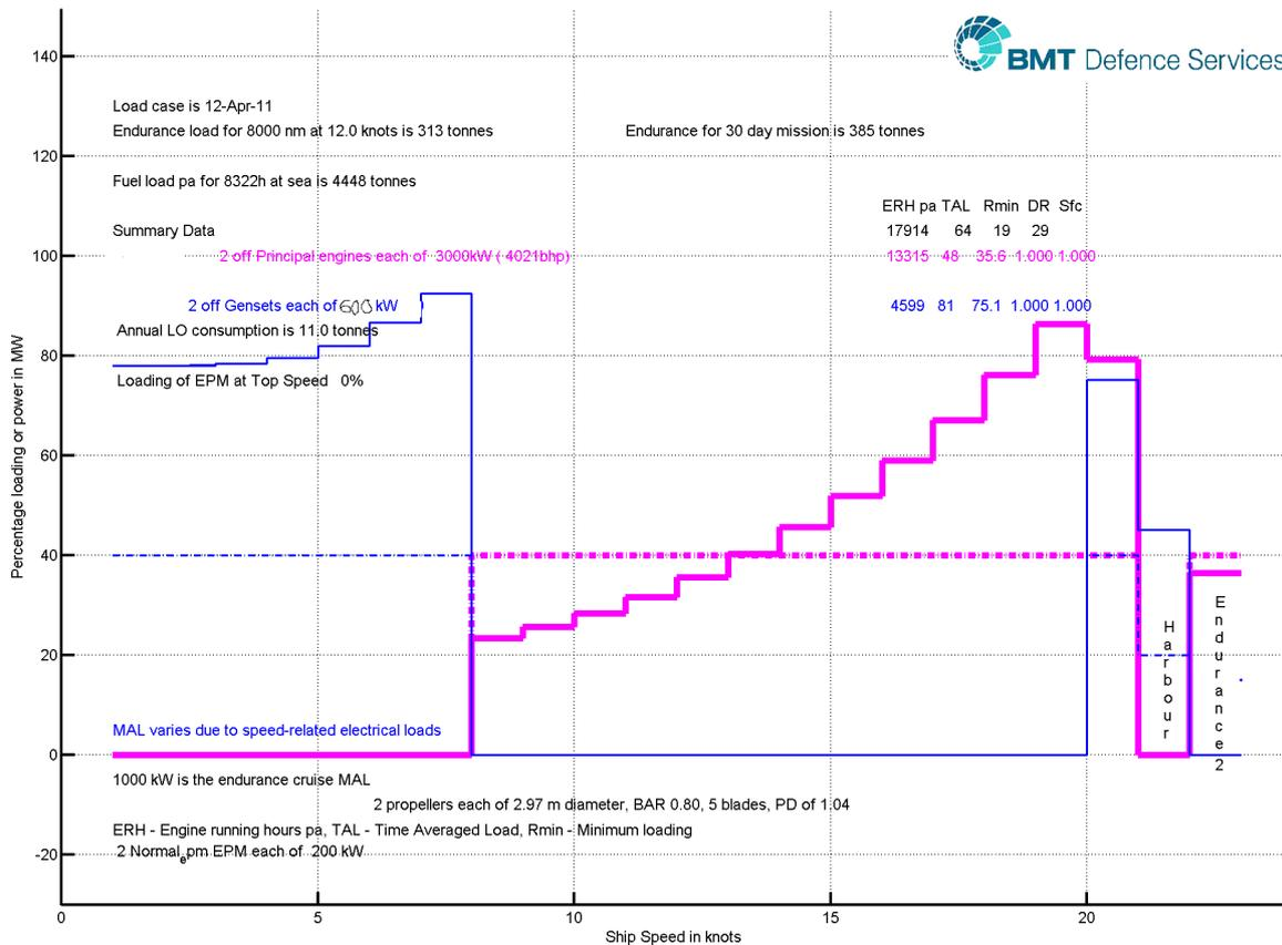
**Figure 4: Hybrid Engine Loadings**
