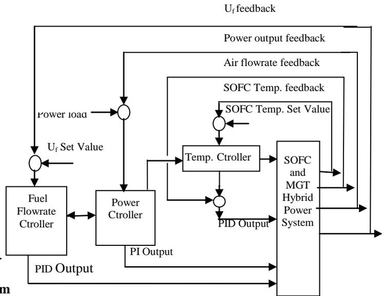
**Figure 3: SOFC-MGT Hybrid Power Control System**
