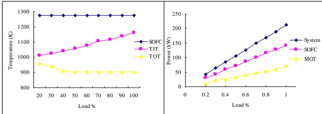
**Figure 5: Temperature of SOFC, MGT TIT and TOT with different power output**
