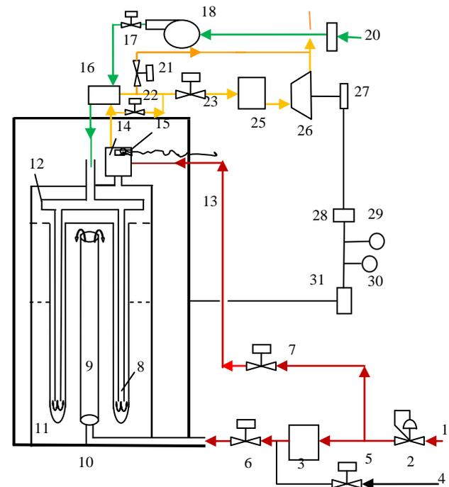
**Figure 1: SOFC and micro gas turbine hybrid system**
