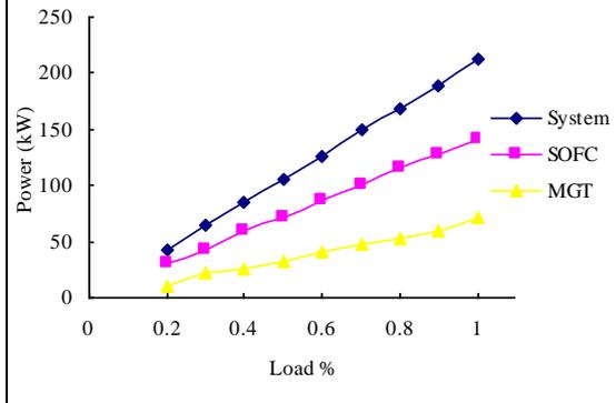
**Figure 6: The hybrid system, SOFC and MGT power output at different load**
