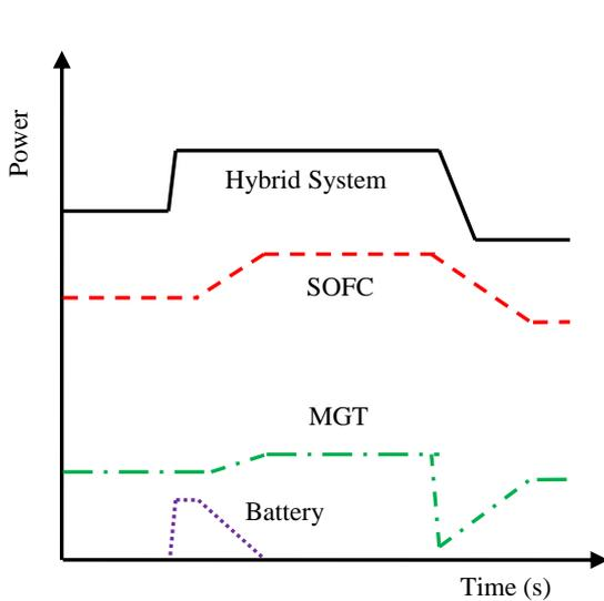
**Figure 2: Power output changes of the system components with the load control strategy**
