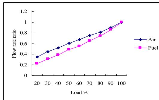
Figure 4: Air and fuel flow-rate vis with power
