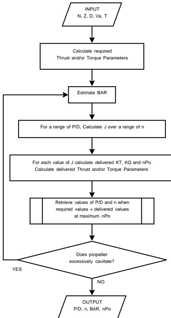
Figure 1: Algorithm for Basis-Propeller Selection.
