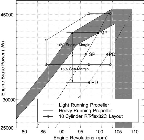
Figure 2: Wärtsilä 10 Cylinder RT-flex82C Main Engine & Propeller Demand Curve for KCS.
