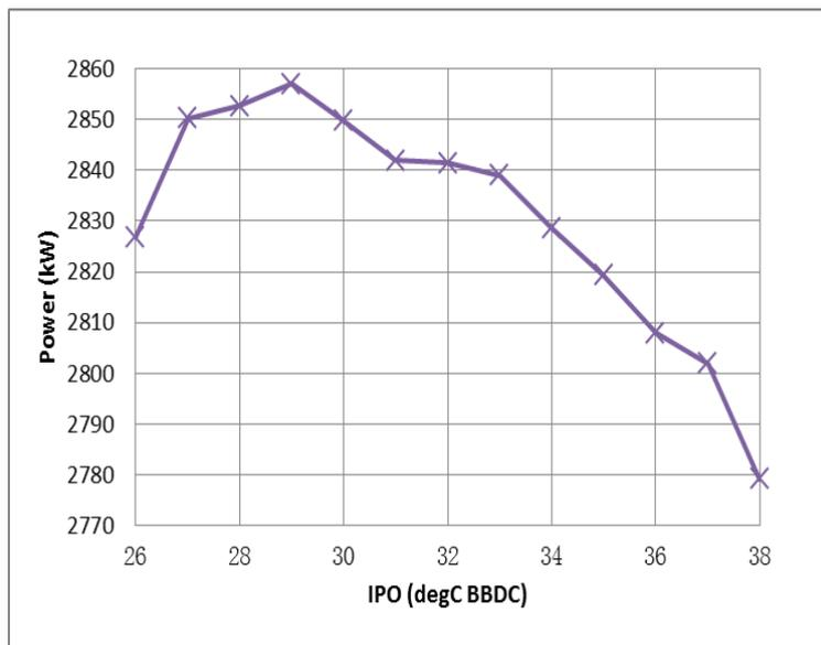
**Figure 15: Intake port opening dependence in engine power optimisation**
