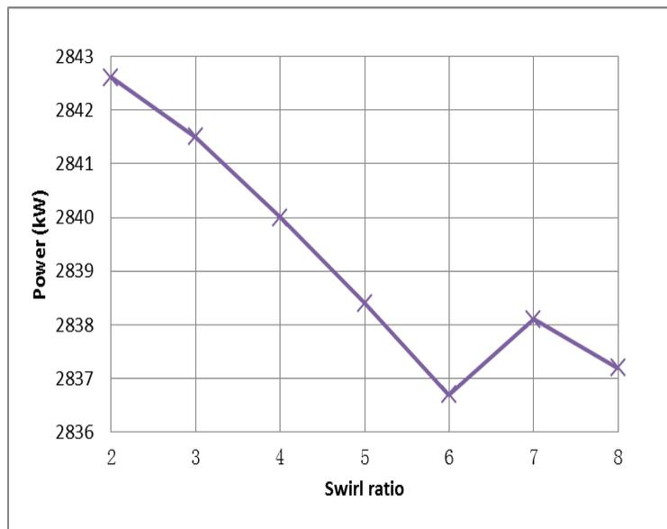
**Figure 13: Swirl ratio dependence in engine power optimisation**
