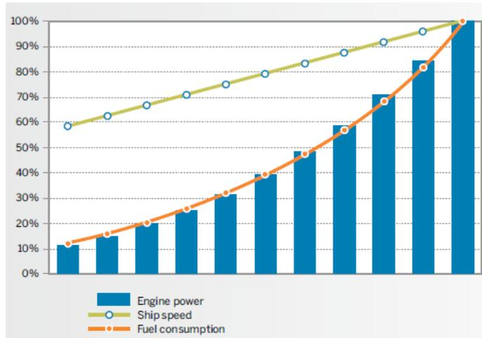
**Figure 2: Correlation between ship speed, fuel consumption and engine power**
