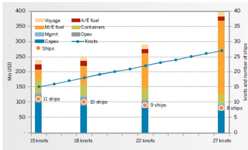
**Figure 3: Operating costs for Europe-Asia service for different ship speeds**
