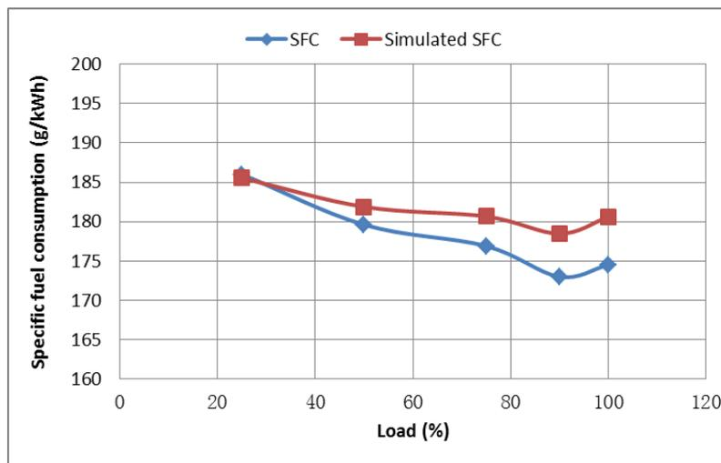
**Figure 4: Comparison of tested and simulated SFC**
