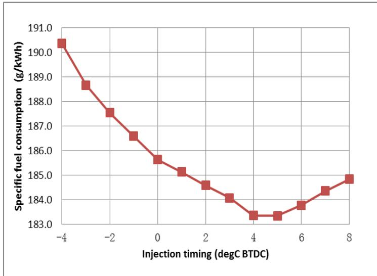
**Figure10: Injection timing dependence in SFC optimisation**
