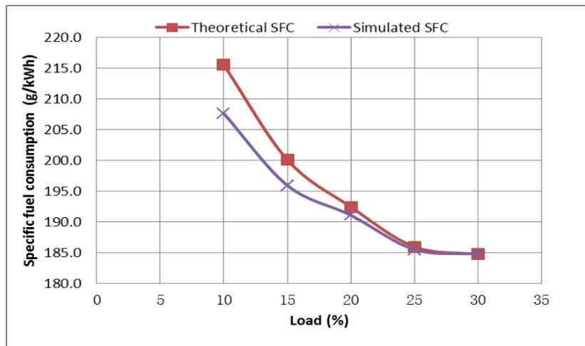
**Figure 8: Simulated engine SFC of ultra-slow speed steaming**
