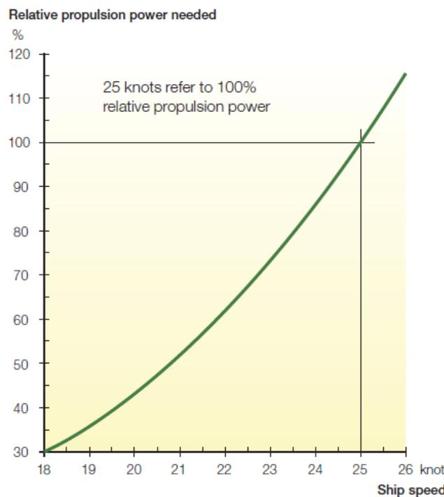
**Figure 1: Required propulsion power for a vessel as a function of speed**
