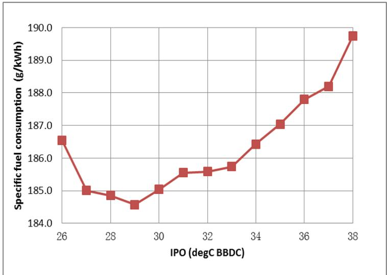
Figure 16: Intake port opening dependence in SFC optimisation
