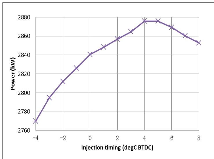
**Figure 9: Injection timing dependence in engine power optimisation**
