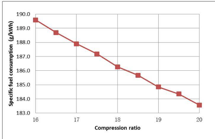
**Figure 12: Compression ratio dependence in SFC optimisation**
