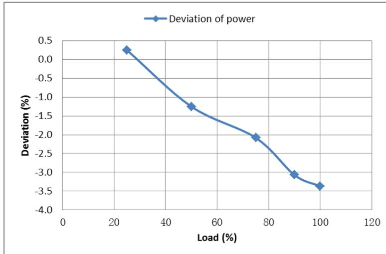
**Figure 5: Deviation of improved simulated engine power**
