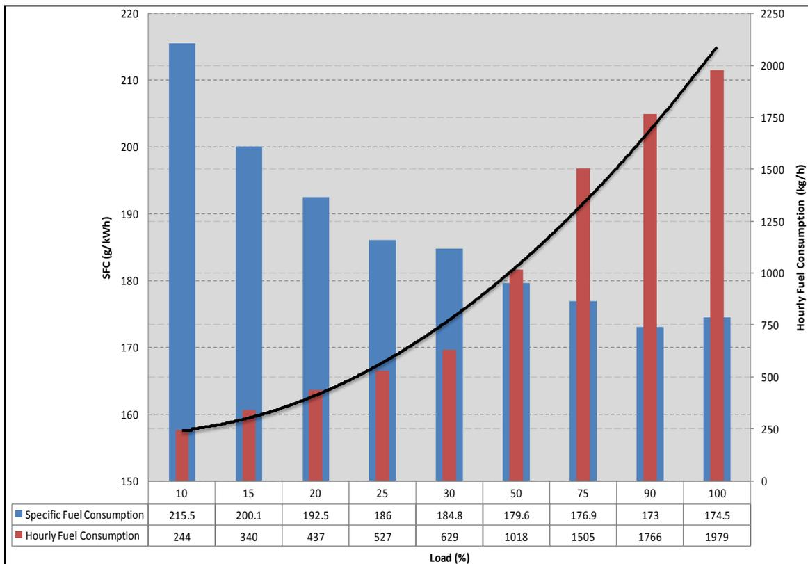
Figure 17: The theoretical SFC and hourly fuel consumption plotted with respect to engine load
