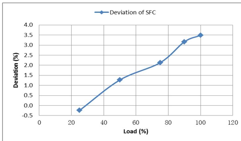
**Figure 6: Deviation of improved simulated SFC**
