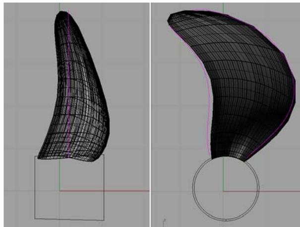
Figure 11: NPT propeller geometry.
