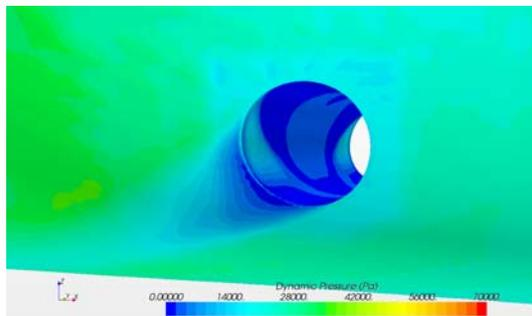
Figure 3 Dynamic Pressure, open thruster tunnel.
