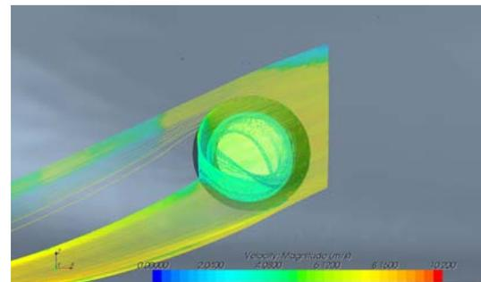
Figure 4 Streamlines, open thruster tunnel.
