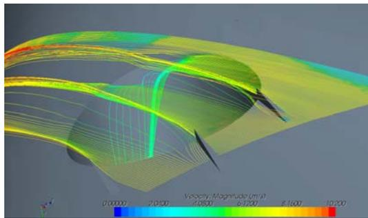
Figure 5 Streamlines, Vortex Generators.
