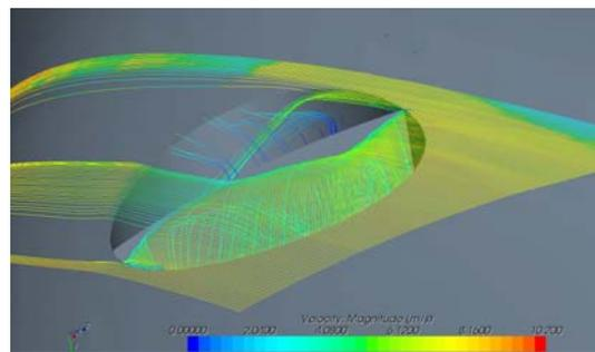
Figure 7 Streamlines, splitter plate.
