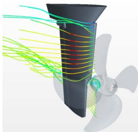
Figure 12 Streamlines in vicinity of the twisted rudder on the gas carrier.
