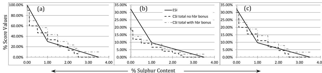
Figure 6. A comparison of SO<sub>x</sub> scores generated by ESI and CSI. (a) Compares % contributions to SO<sub>x</sub> component of each index. (b) Compares % contributions to the total of the respective indexes. (c) Compares % contributions to the emissions components for the case of the CSI.
