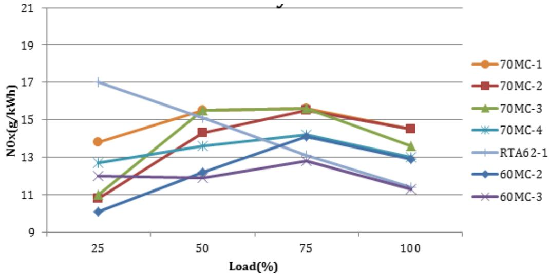
Figure 8. Exhausted NO<sub>x</sub> at each load (E2 Cycle)
