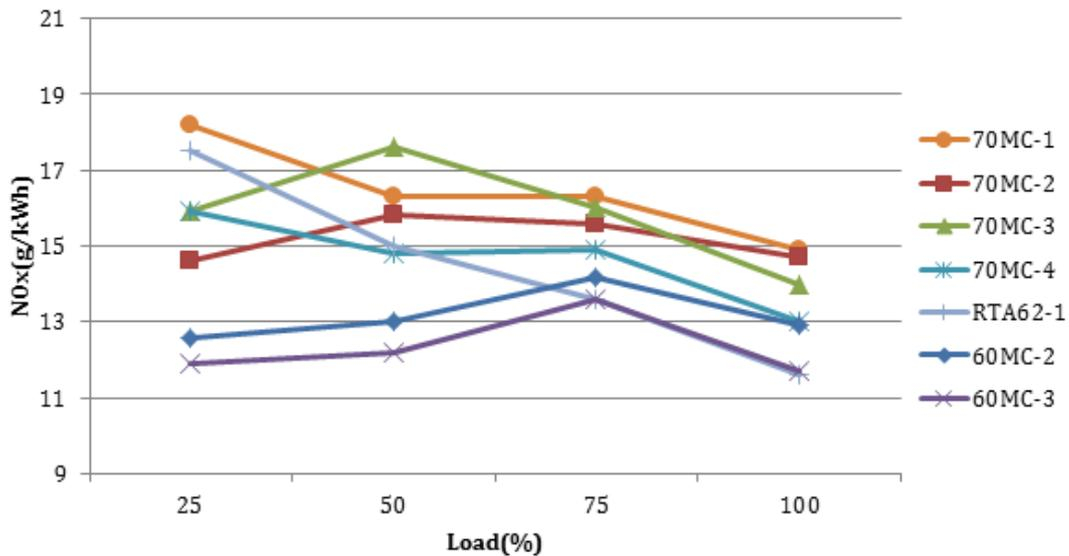
Figure 9. Exhausted NO<sub>x</sub> at each load (E3 Cycle)
