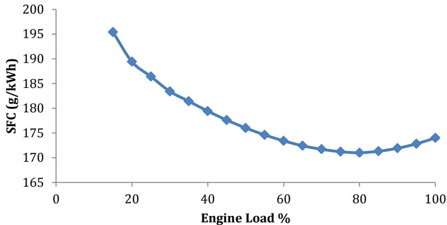
Figure 7. Specific Fuel Consumption of MAN engine (6S70MC-C)
