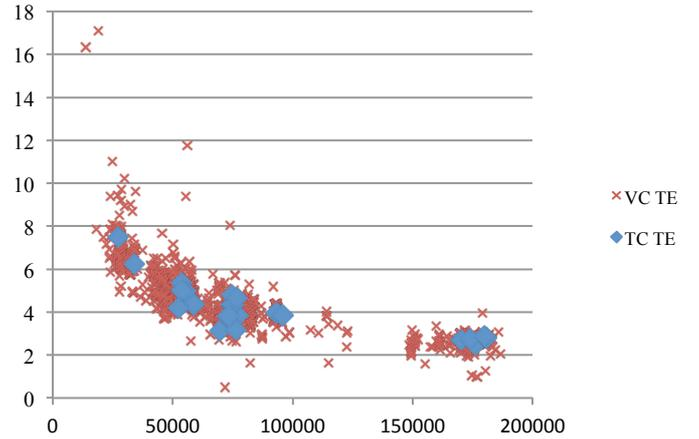
**Design vs. Operational speed ratio comparison for wetbulk**
