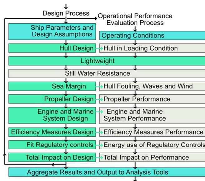
Figure 1: Functions in the (steady-state) Whole Ship Model.
