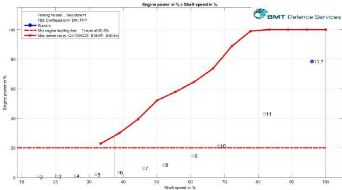
Figure 2: DM FPP drive: Engine characteristic
