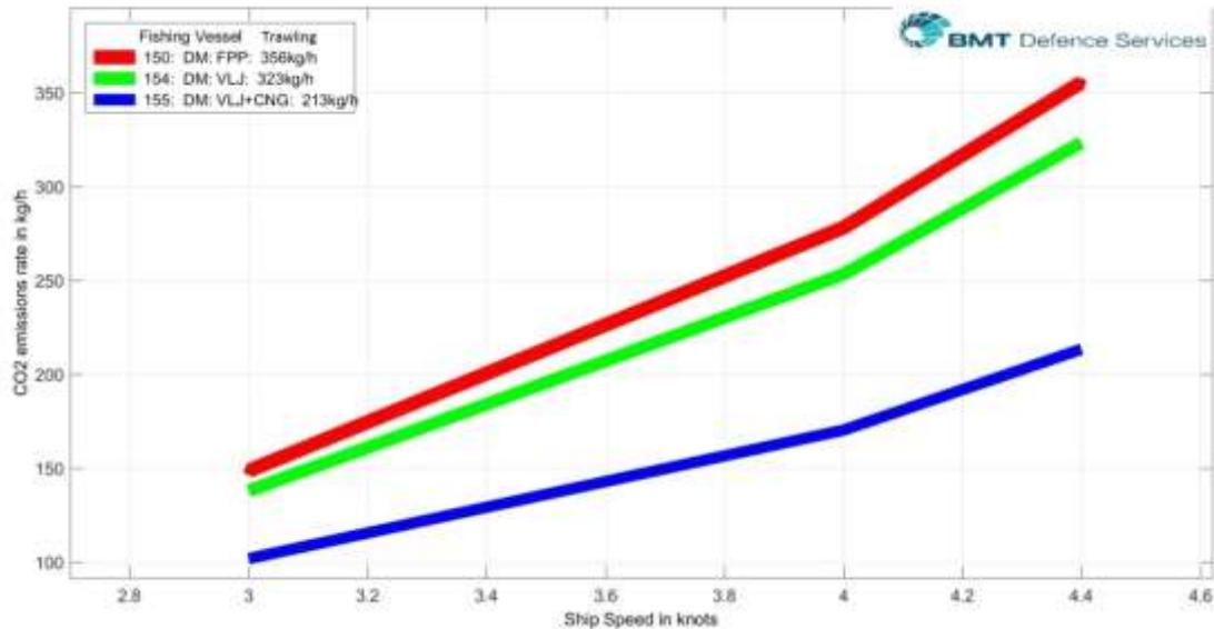
Figure 8: CO<sub>2</sub> emissions when trawling
