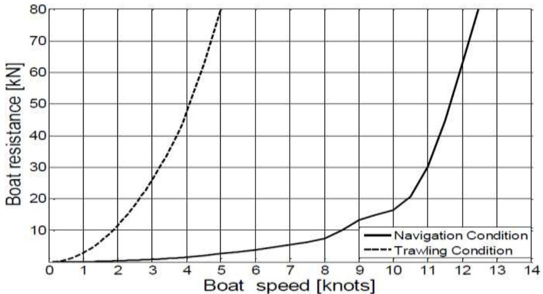
Figure 1: Vessel resistance in navigation and trawling conditions.
