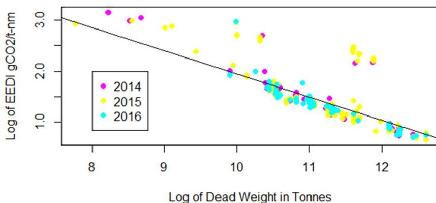
Figure 2 showing the natural logarithm of verified EEDI of vessels against the natural logarithm of dead weight in tonnes by year,  $n = 615$   $p$  value 2.2-16, negligible, which is a result of the EEDI methodology and is to be expected (Canning T. M., 2016).
