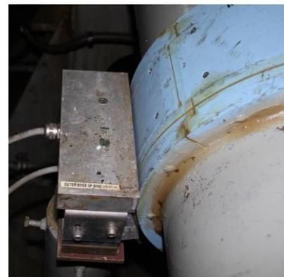
Figure 3 Shaft power meter
