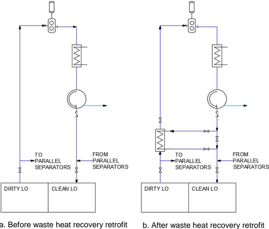
Figure 4: Heat Exchanger Retrofit into Purification System
