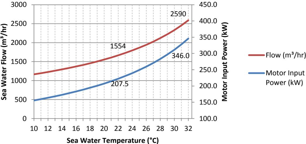
Figure 2: Demonstration of Opportunity for Variable Sea Water Flow against Sea Water Temperature
