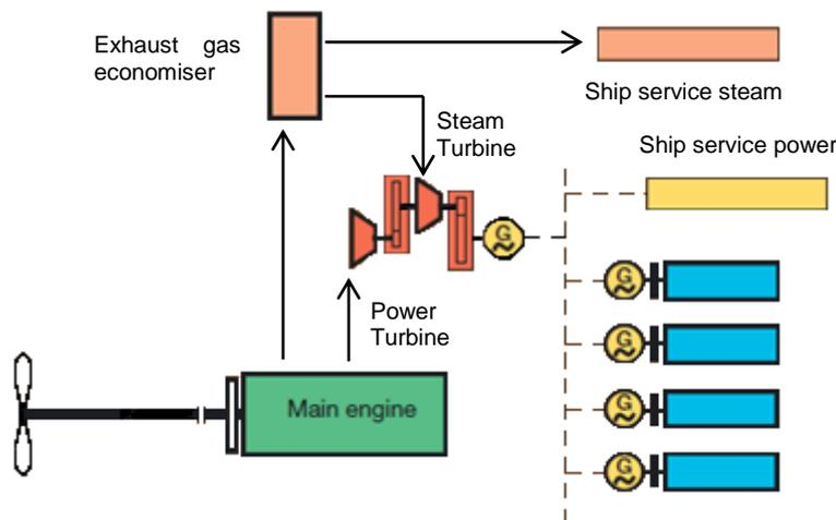
Figure 1: Example Waste Heat Recovery Plant Arrangement
