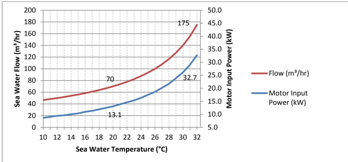
Figure 3: Variable Sea Water Flow against Sea Water Temperature for Nominal Chilled Water Plant load of 750kW
