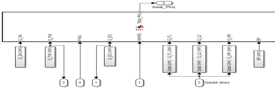
Figure 7 Heat balance of two stroke LSDE as part of MEP energy model
