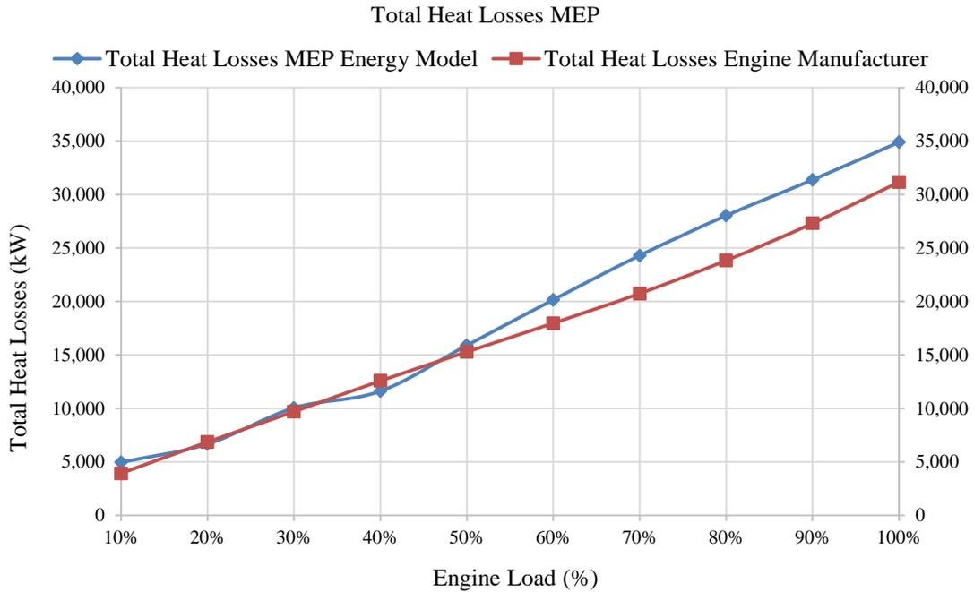
Figure 8 Total heat losses MEP
