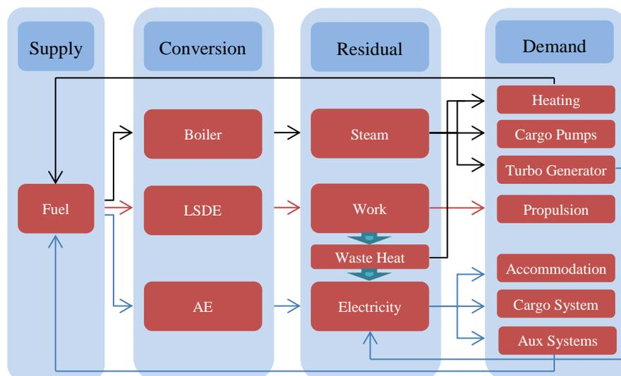
Figure 4 MEP's algorithm of operational condition and conversion systems
