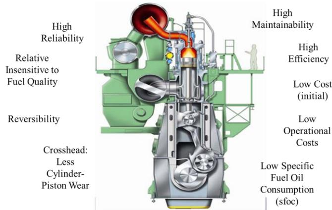
Figure 2 Sectional view and advantages of two stroke LSDE (MAN, 2013b)
