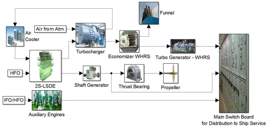
Figure 3 Common MEP configuration of existing VLCCs
