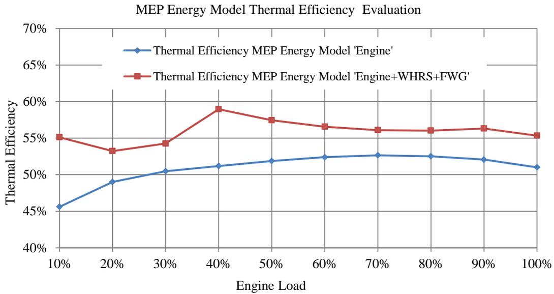
Figure 9 MEP energy model thermal efficiency evaluation
