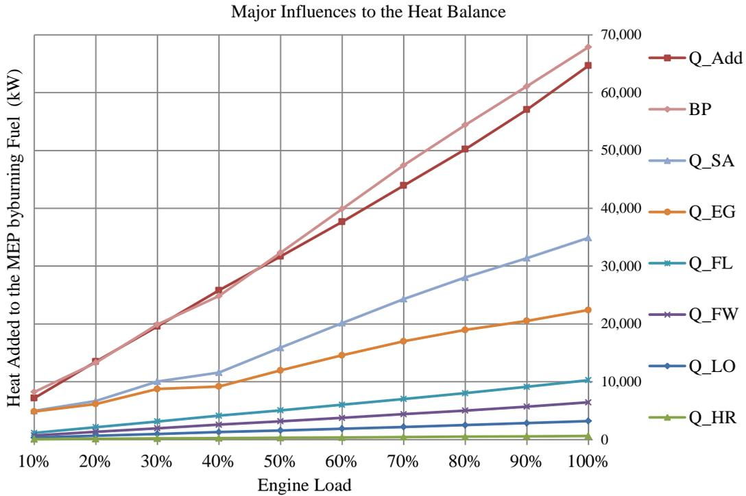
Figure 10 Heat balance of the engine of the MEP energy model
